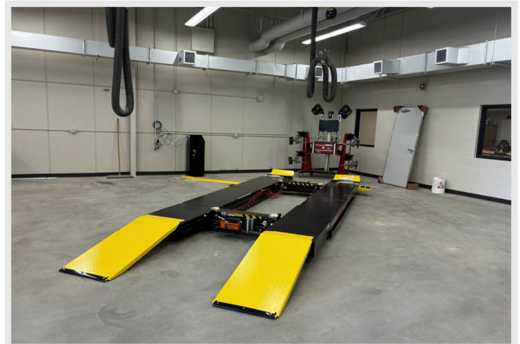
The new 14k scissor lift installed and powered up in the Auto Shop. Looking good!
